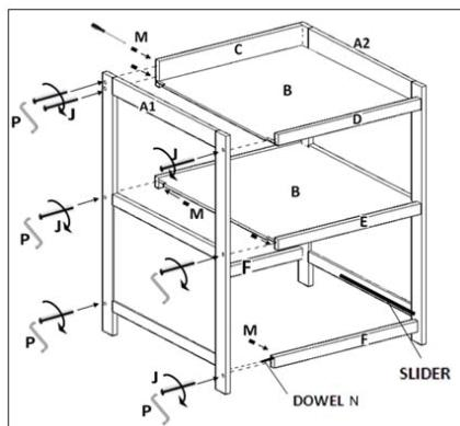
**Step 1 :** Use the right legframe **A2**, the shelves **B**, the back **C**, the crossbars **D-E-F**, seven bolts **J**, seven cylindrical nuts **M**, four wooden dowels **N** and the hexagonal key **P**
